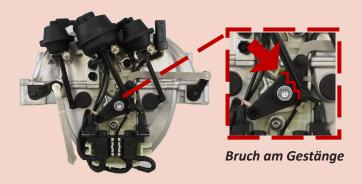
Due to the interaction between thermal stress, vibration and the escaping oil, the plastic material of the linkage becomes porous and breaks.
