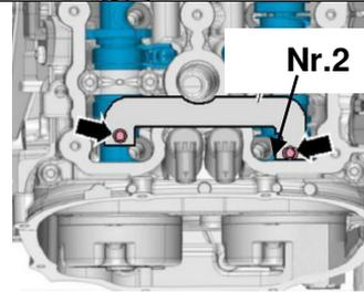
Push back the timing chain tensioner and fix it with the tool No.3.
