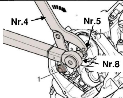
Hold the camshaft sprocket with two-pin wrench No.4 and loosen the camshaft sprocket.
