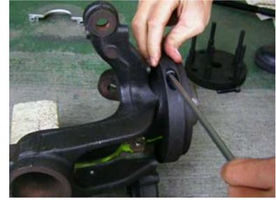
Hammer the bolts (3) carefully into the mounting plate – the bolts (3) have to be aligned with the wheel hub's hole circle.
