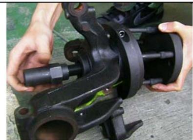
Pull out the worn out wheel hub/bearing unit with the spindle (1) and the spindle nut (8).
