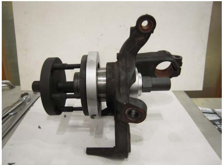
Pull in the new wheel bearing with the bearing spindle (1) and the spindle nut (8).
