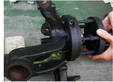
Attach the dismantling plate (7) sideways to the drive shaft and lead the spindle (1) with the attached mounting plate (2) from the front through the wheel hub and the dismantling plate (7).
