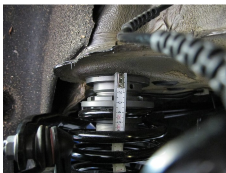
Pic 2: RA spring plate adjustment dimension
