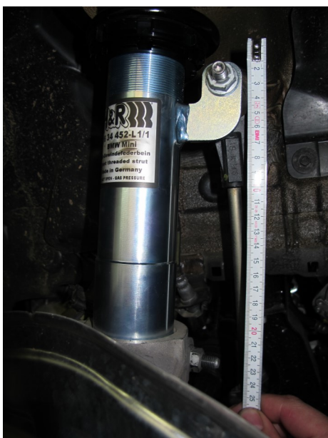
Pic 1: FA spring plate adjustment dimension
