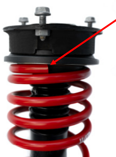
Bild 3: Position Federende beachten Fig. 3: Mind correct position of the spring end
