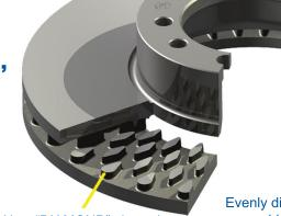
New "DIAMOND" shaped pillar vent to substantially increase airflow Evenly distributed vents giving greater support to the braking surface, reducing the risk of high spots
