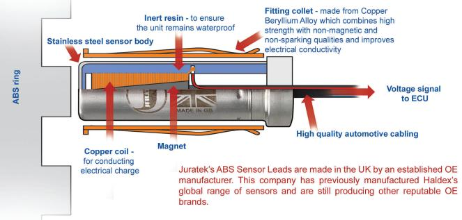
All our sensors are tested 10 times throughout the manufacturing process. Then 10 random test samples are selected from every batch. These are then subjected to harsh bump and environmental tests to emulate the harsh conditions of being on the road. It is only when all tests are complete, that each batch are released for dispatch.
