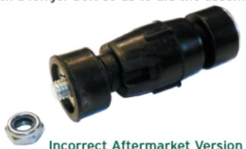
The Original Equipment version has the correct length of bolt for a reason. The stabiliser bar and suspension arm need to be compressed so as to allow the nut to be fitted. This is done to apply the correct torsional load. If the stabiliser link is not correctly compressed / tightened this cannot be achieved.
