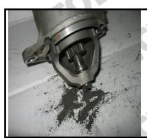
Signs of grey/metal dust can indicate that failure of the starter motor has been caused due to a failing Dual Mass Flywheel.
