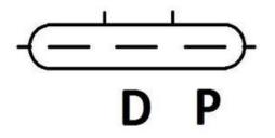
This alternator is externally regulated through the vehicle ECU and the voltage is controlled by the ECU.
