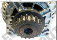
Uneven wear marks caused by incorrect fitting of alternator.
