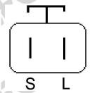
AEA2238/AEK2314 - This alternator is internally regulated. The charging process is controlled by the alternator. This alternator can be identified by testing the wires on the wiring harness to the alternator. The 'S' terminal should show a permanent battery voltage and the 'L' terminal should show voltage with the ignition switched on. This part is also commonly affected by burnt/rusty pulleys or belt slip. Please inspect you old unit for signs of this failure and ensure the belt is replaced.
