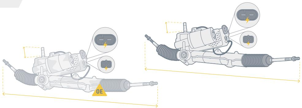
Compare the old and new steering rack – are they physically identical? Is the length correct? Compare threads on inner tie rods and mounting threads. Is the pinion correct – both in size, shape and position?
