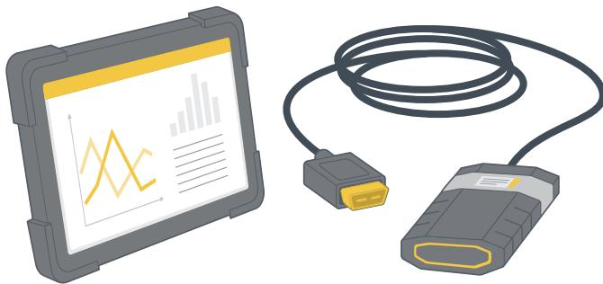
Before starting disassembly, error codes related to the steering rack must be deleted if possible.
