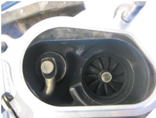
Gasket incorrectly mounted
