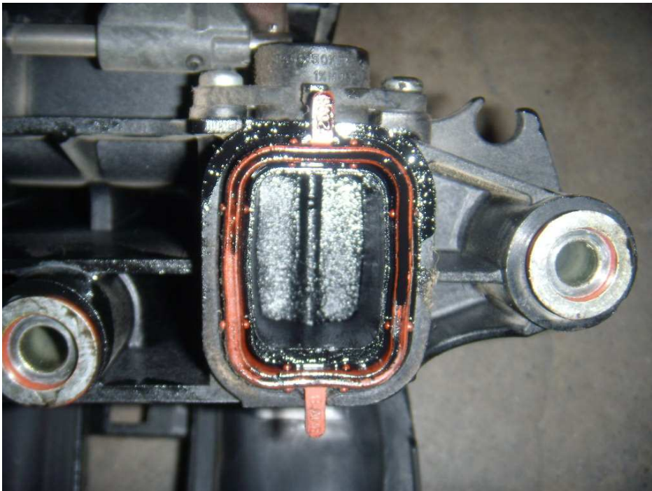
Plastic air intake manifold with additional swirl flap
