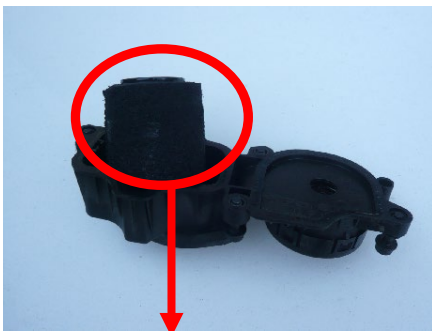
BLOCKED NON FUNCTIONING FILTER.
