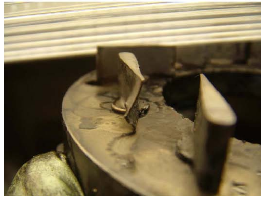
Damaged nozzle blades.
