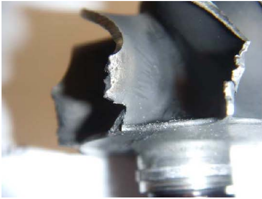
Damaged exhaust turbine
