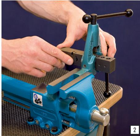
Then push the gripping jaw (3) into the basic unit (2) so that the side with the inscription „180°“ (on older gripping jaws the inscription is „F“) faces upwards.
