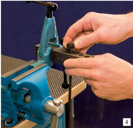
Plug the pressure piece, which has been made slippery and corresponds to the tube diameter, onto the tube. Place the base block (5) on it with the opening facing downwards. Then push the gripping jaw (3) into the tool until the tube end with the thrust block and base block (5) is under the pressure spindle.
