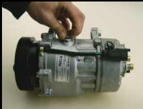
7. Put drain plug back into compressor.
