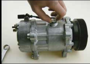
1. Loosen drain screw for oil care 2. Turn out drain screw completely
