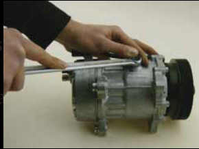
1. Loosen drain screw for oil care 2. Turn out drain screw completely
