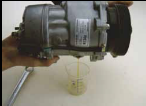
4. Empty compressor completely, turn clutch therefore releasing the oil
