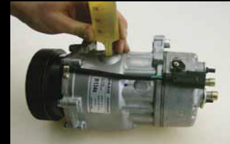
6. Adjust oil quantity according to manufacturer's advice
