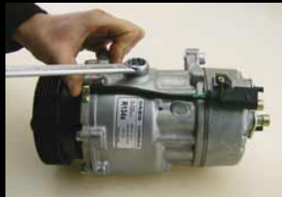
8. Tighten drain plug (but DO NOT over tighten).
