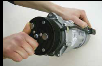
9. Turn the compressor 10 times to distribute the oil.
