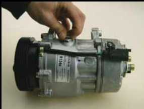
7. Put drain plug back into compressor.
