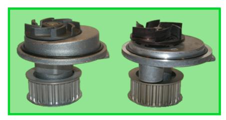
Viewed in profile the depth of the latest design pump is clearly much shallower than FWP 1575, and care should be taken to ensure that the pump is correctly located in the engine block.
