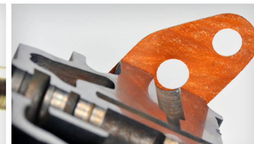
Incorrect shape and position of gasket
