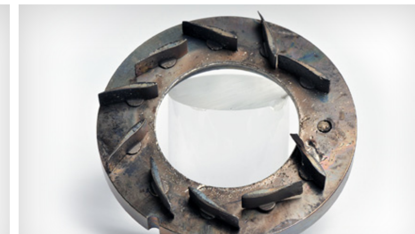
Damage to a nozzle assembly
