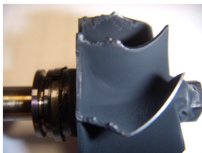
Damaged exhaust turbine
