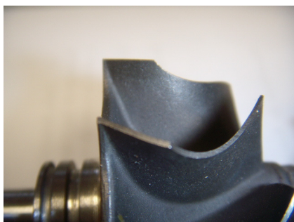
Undamaged exhaust turbine
