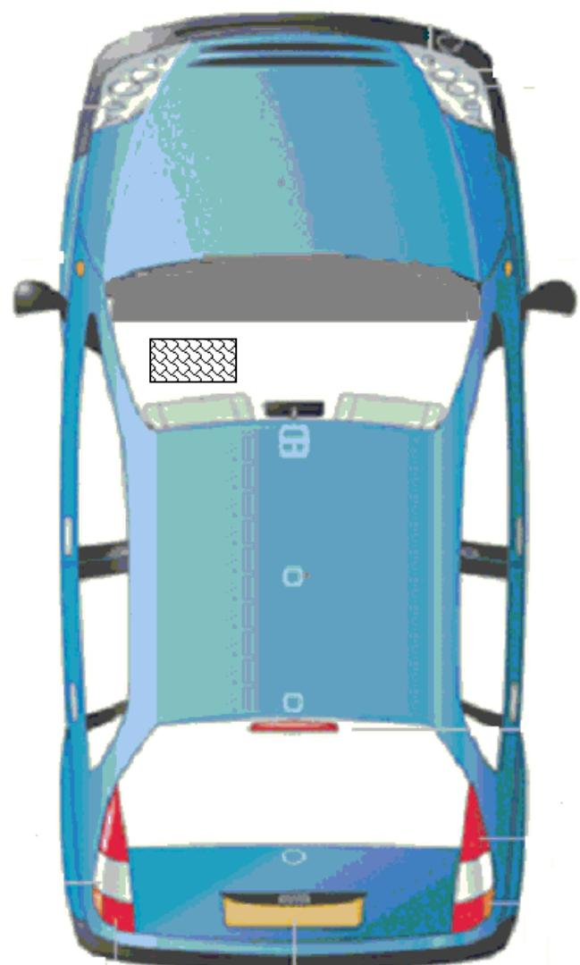
1. The Cabin Filter can be found in the passenger's footwell underneath the glove compartment.
