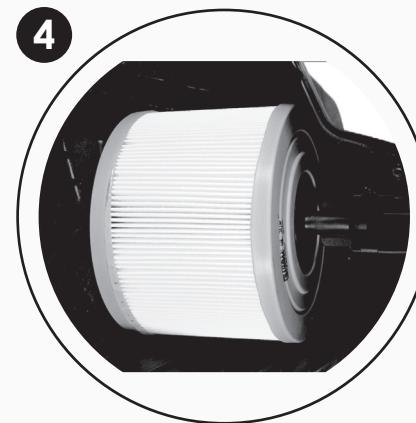
**GB** Properly installed filter (pictured). Close and fasten the housing cover.
