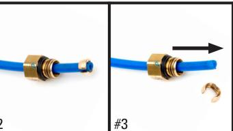
NOTE: SCRATCHES AND/OR DEEP CUTS IN THE AIR LINE CAN RESULT IN POSSIBLE LEAKS. INSPECT THE AIR LINE BEFORE INSERTION. AIR LINE NEEDS TO BE REPLACED IF DAMAGED.
