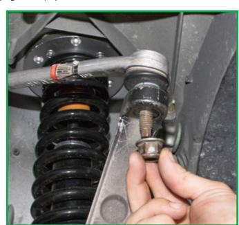
4. Install sway bar end link bolt and nut. (Figures 10, 11)
