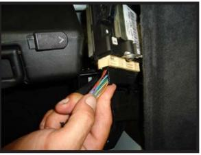
FIGURE 1A 2. Remove both plugs located on the control module. (FIGURE 1B)
