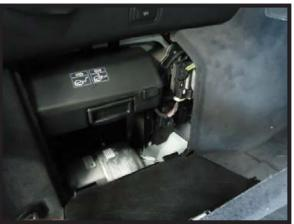
FIGURE 1B 3. Remove the cover of the larger plug by sliding it off of the end. (FIGURE 1C)
