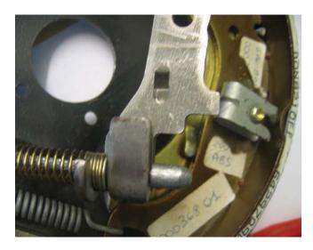
2. The outer spring sleeve is placed as shown and then the lever is crimped as shown to complete the assembly.
