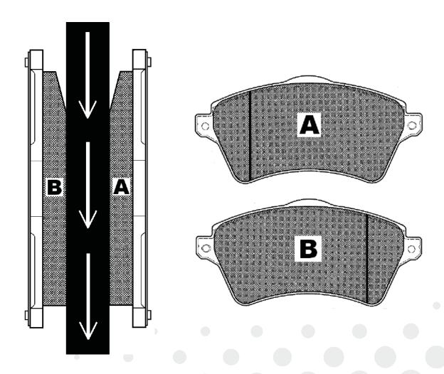
Due to the design of the braking system found on this vehicle, it is imperative that the replacement brake pads are fitted as shown above.
