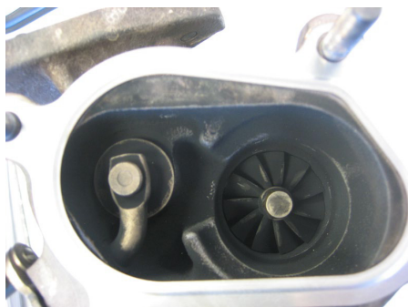
Gasket incorrectly mounted
