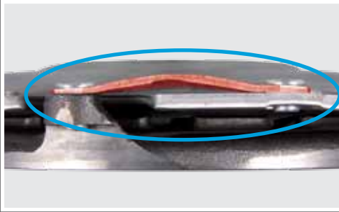
Bent tangential leaf spring
