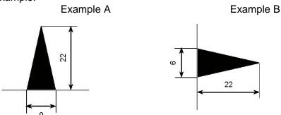
After 10 Minutes the sag shall be measured. The horizontal bead, Example A, shall not sink by greater than 3mm and the vertical bead, Example B, shall not droop greater than 3mm from the centre line.
