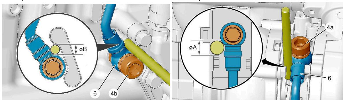
*Pay attention for the correct assembly like illustration (D), the pipe has to go through the center line of the connection (E & F)*
