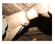
Original dust cover with smaller drain-hole
