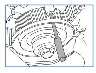
Pin 'C' is used twice during the timing belt replacement process, and is used to align both the crankshaft and injection pump sprockets.
