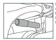
Pin 'A' is used to lock the crankshaft by locating in the back of the flywheel, allowing the crankshaft bolt to be loosened/re-tightened.
