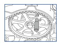
Pin 'B' is used to locate the amshaft sprocket and ensure it does not move during timing belt removal and installation.
