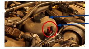
On removal of the engine cover, you will find the oil filter element housing in the centre of the engine at the top.
