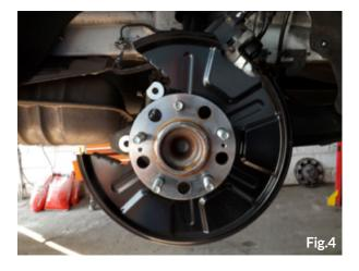
10. Finally, rewind the EPB motors and check the operation of the parking and foot brakes, which includes checking for fluid leaks. Then recheck for fault codes in the EPB and ABS systems, refit the wheels and torque wheel nuts to 88-108 Nm and road test.
