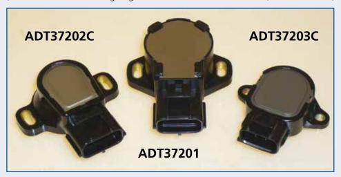
This device signals the exact position of the throttle valve at any time to the engine ECU by varying the output voltage through a variable resistor or potentiometer. It is a key component in the vehicle engine management system and if malfunctioning may cause symptoms such as;
