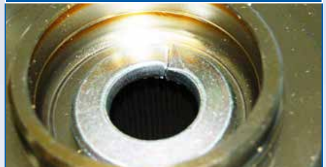
Correct position of washer
