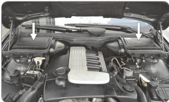
Open the front bonnet, the pollen filters are located symmetrically on both sides in rectangular housings
