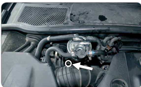
(EN) Loosen damping ring fastening the filter, remove filter
