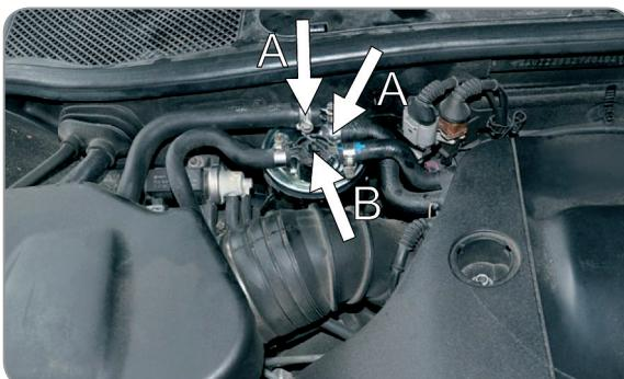
**(EN)** Fix fuel hoses (A), regulation valve and clamp fastening the valve (B). Start the engine, check for leakage
