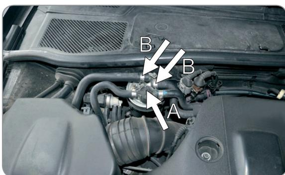
(EN) Remove fastening clamp and regulating valve (A), loosen fuel hose bands, remove hoses(B)
