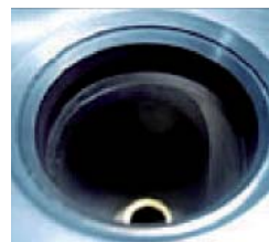
Figure 6: The optimum fitting result with replaced valve seat insert.
