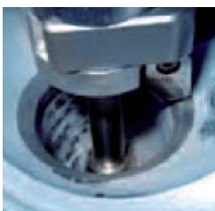
Figure 1: Removing the valve seat insert by milling.
