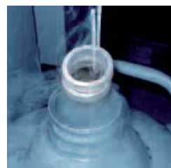
Figure 4: The valve seat inserts are cooled down in liquid nitrogen to facilitate fitting.
