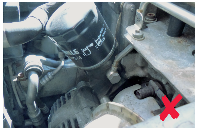
Figure 3: Depending on the installation position, it is important to keep oil from entering the alternator during oil changes.
