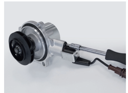
Figure 3: The new, uncontrolled coolant pump with reattached actuator
