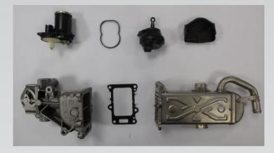
All components are stripped, cleaned of carbon deposits, inspected for wear, and replaced where necessary.
