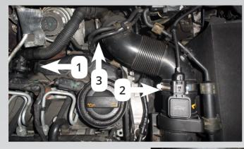
Remove particulate filter and downpipe\* Disconnect crankcase breather hose (1) Detach air pipe from air filter housing (2) Move air hose and connection to rear and detach from turbo charger (3).
