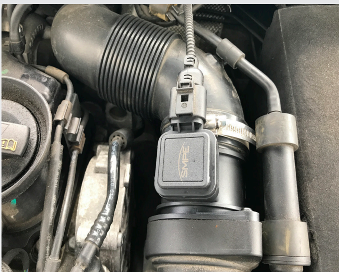
Check Inlet for Leaks
