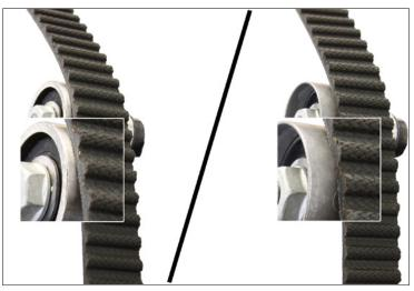
Image 2: Deflecting pulley 532 0623 10 (left)/deflecting pulley 532 0349 10 (right)
