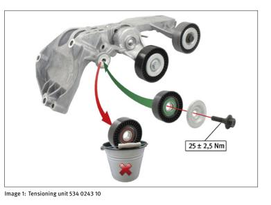
The tensioning unit assembly is fitted as standard with deflection pulleys that are suitable for petrol engines only.
