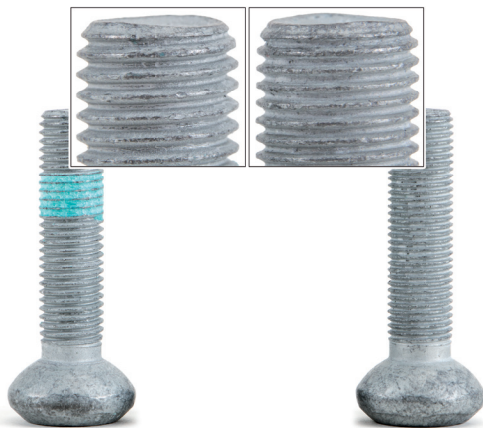
Fig. 1: Left screw: M12x1,5 Right screw: M12x1,25
