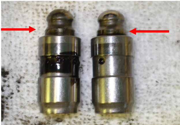
Bild 3: Left: hydraulic lifter is extended to the maximum, seal valves. Do not replace lifters!
