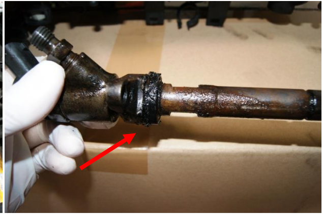
Bild 2: Re-seal the leaking holding bracket of the injection nozzle
