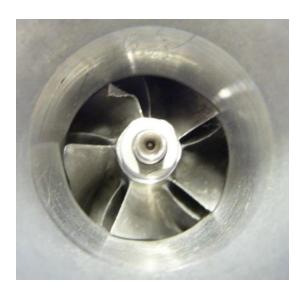
If one of the vanes of the compressor wheel is bent (see picture) the complete suction area should be checked and cleaned.
