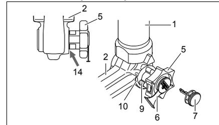
**Odjištěná poloha, odpojeno**
